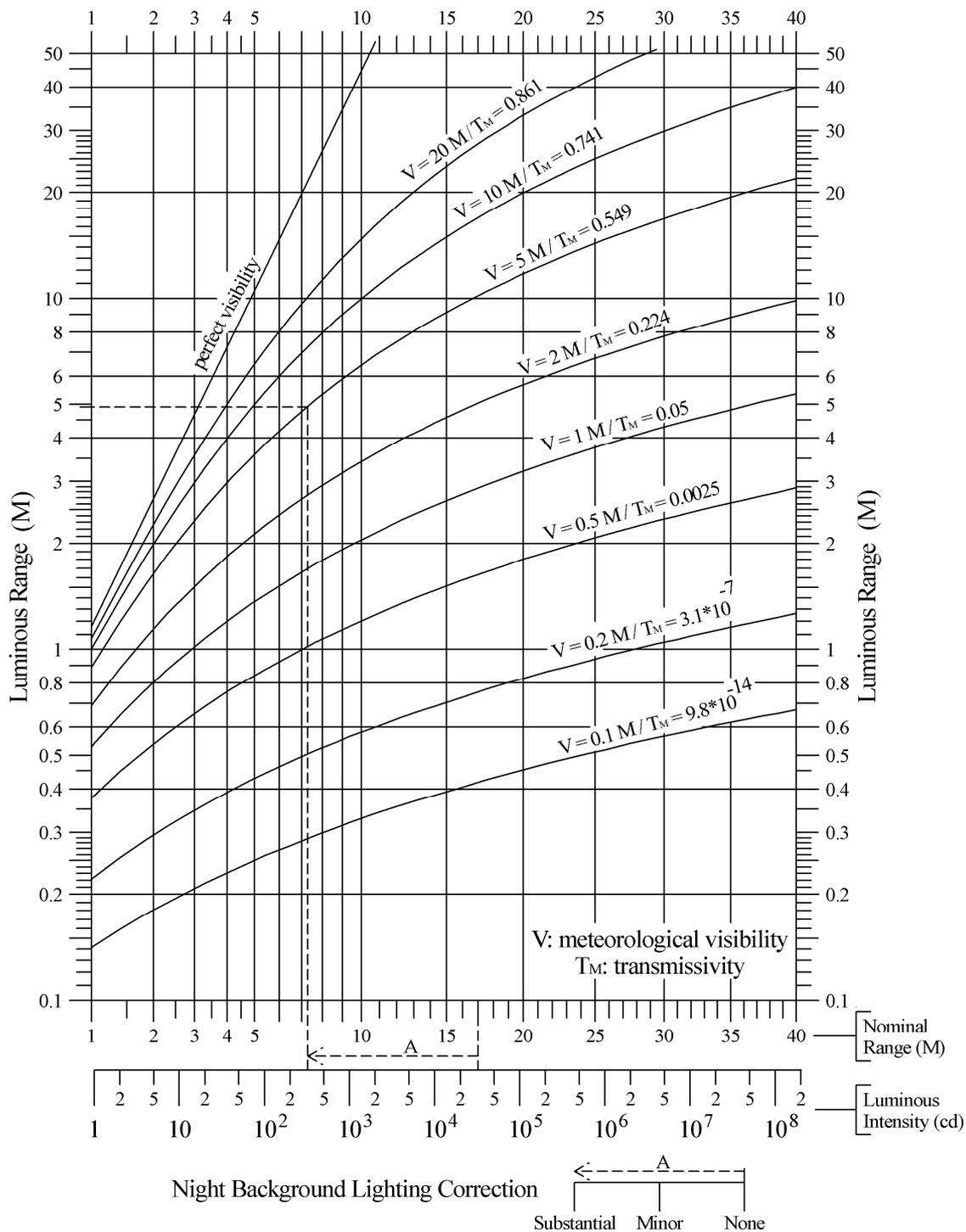
Figure 2 Luminous Range diagram – night time
